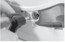
2. Connect the AC power cord to the AC power
